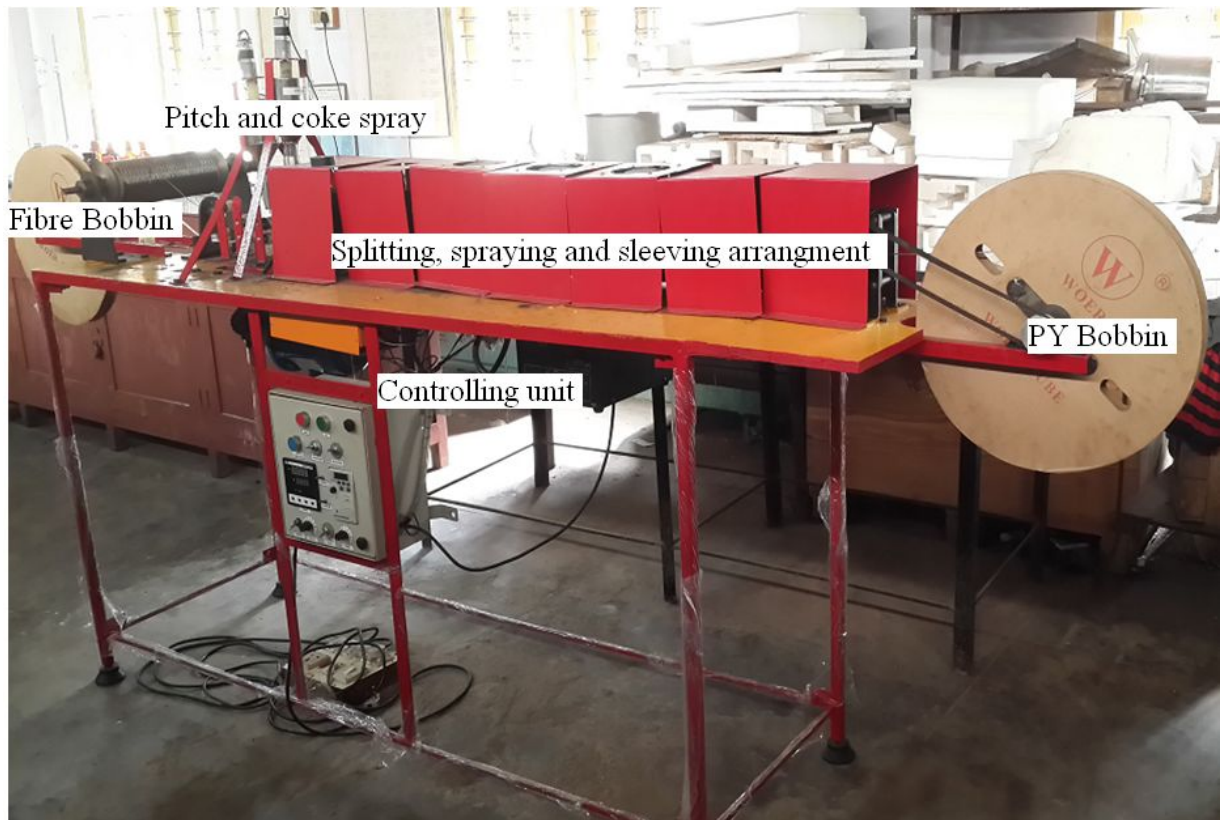
Fig. 4.41 Photograph of final PY machine with splitting, spraying and sleeving arrangement
