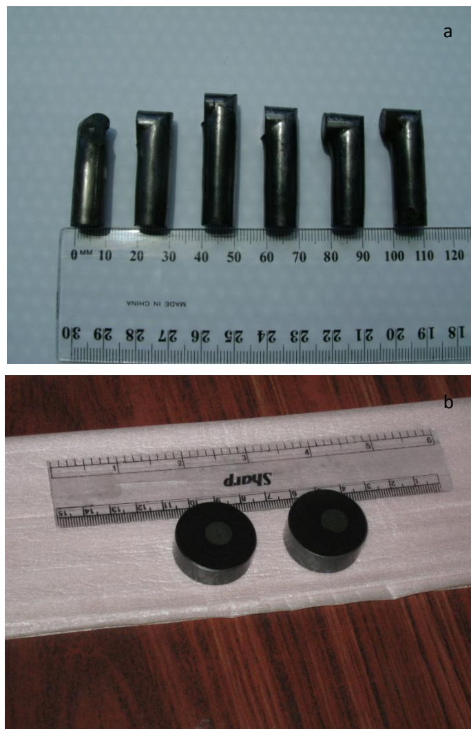
Figure 5.11 a) ECAP-BP consolidated pellets, b) Portion of the pellet hot mounted on polyfast for various analyses
