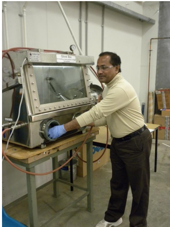
Figure 2.7 operation of glove box in an evacuated mode
