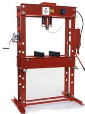
Figure 3.3 Hydraulic press (50 ton capacity) located at the metal powders laboratory at ITRI, Deakin University, Waurn Ponds, Geelong, Victoria, Australia.
