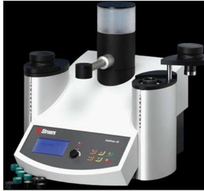
Figure 3.12 Hot compression mounting equipment along with resin mounted samples.
