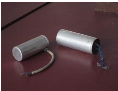
Fig.4.13 Power Capacitors used for testing.
