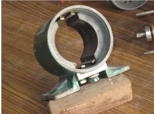
Fig. A.V.5 Stator of PMDC motor showing the poles.
