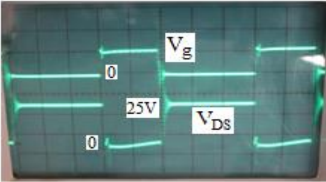
Fig.4.38 MPPT converter waveform: "Time vs. Gate voltage ( V_g ) and Voltage across MOSFET ( V_{DS} ).
