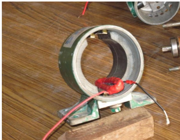
Fig. A.V.6 Stator of PMDC motor showing field coil.
