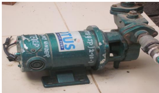
Fig. 4.36 Solar pump used for experimentation.
