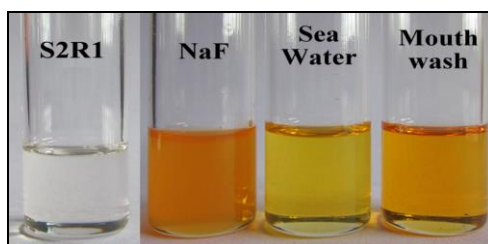
Fig 3.18 Receptor S2R1 showing colour change upon addition of NaF, seawater and commercial mouthwash
