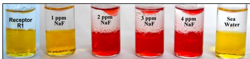
Fig. 7.17 Extraction process of F^- ions from aqueous solutions and sea water using receptor S6R1 solution in DCM
