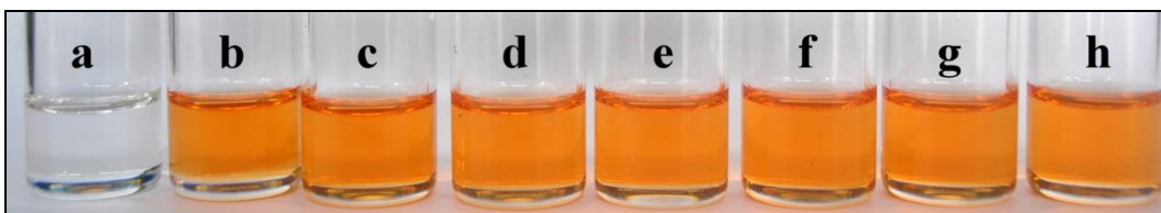
Fig. 3.11 S2R1 solution ( 2.5 \times 10^{-5} M) in DMSO after adding 1 equiv. of TBAF and 1 equiv. of other anions; (a) Free S2R1 , (b) F^- , (c) Cl^- + F^- , (d) Br^- + F^- (e) I^- + F^- , (f) NO_3^- + F^- , (g) HSO_4^- + F^- and (h) H_2PO_4^- + F^-
