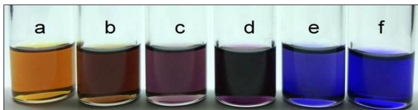
Fig. 4.14 Colour change of S3R1 with varying composition of DMSO in DCM on adding F^- ions; (a) 0% i.e. 100% DCM, (b) 20%, (c) 40%, (d) 60%, (e) 80% of DMSO in DCM and (f) 100% of DMSO
