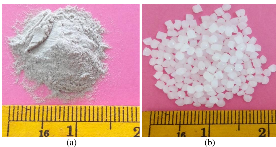
Figure 2.1 (a) Cenospheres and (b) HDPE matrix used in the present work.
