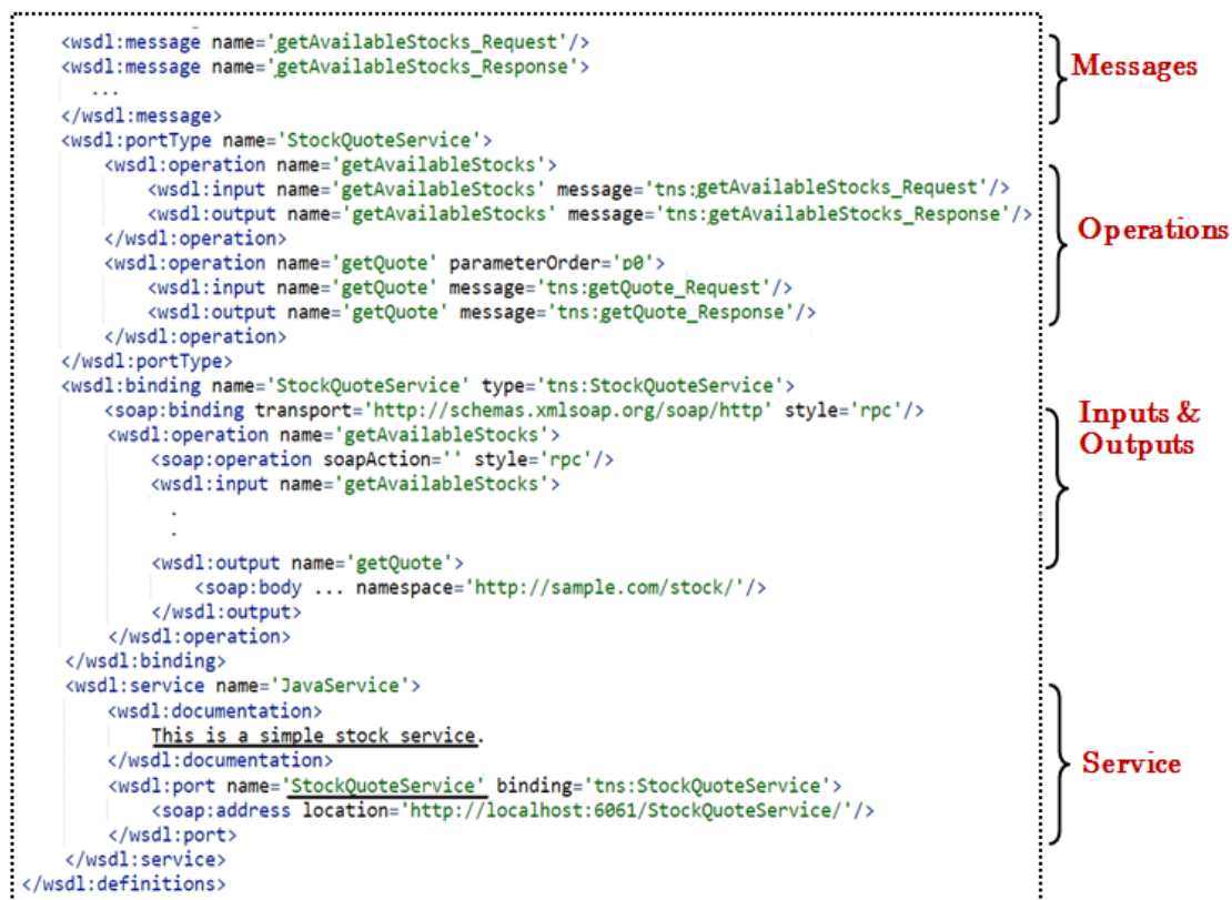
Figure 5.2: A sample WSDL and its functional elements
