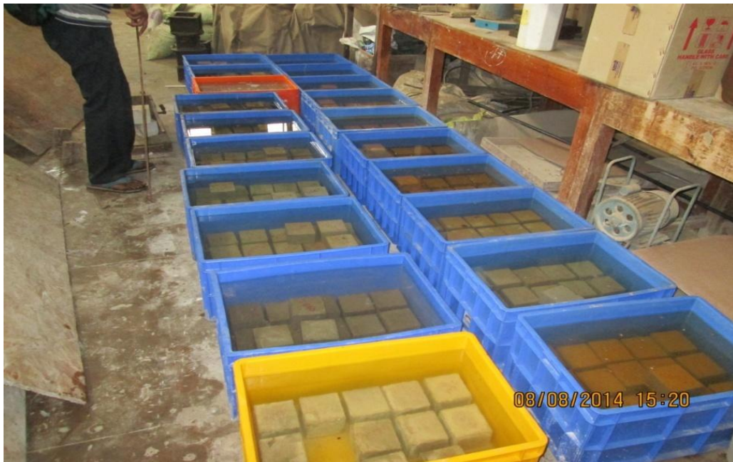
Fig. 3.6 Immersion of cubes in plastic containers for durability tests
