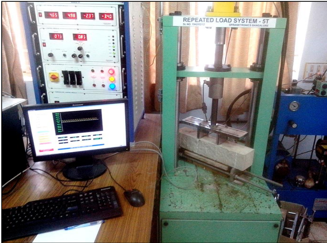
Fig. 3.7 Repeated load testing set up
