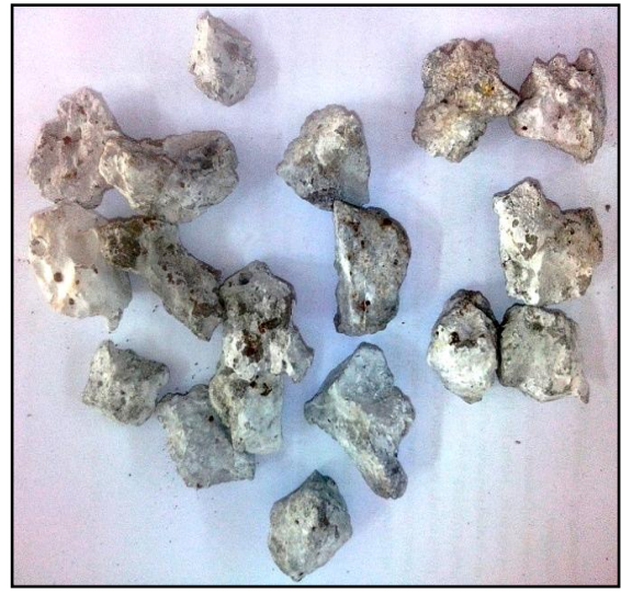
(b) Formation of thin film of calcite on slag aggregates after weathering process
