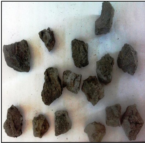
(a) Steel slag aggregates before weathering process
