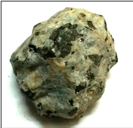
(c) Enlarged image of steel slag aggregate showing coating of calcite
