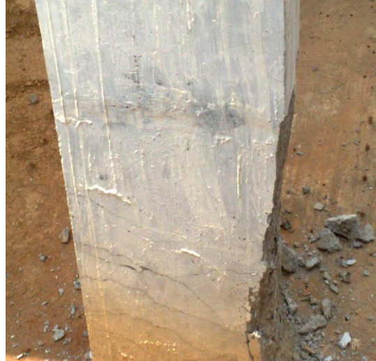
Fig 3.14 Failure mode of CL 20
