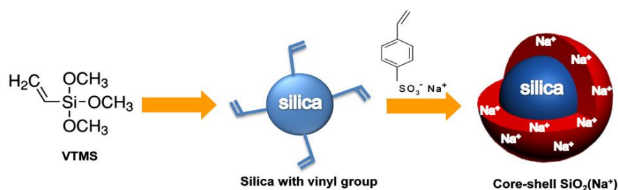
Figure 1.9 Core-shell structured SiO 2 nanoparticles containing poly(sodium 4-styrenesulfonate)
