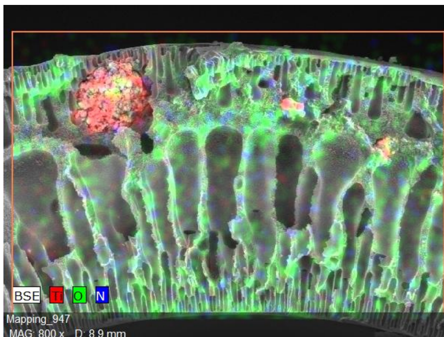
Figure 6.5 Elemental Mapping of P-1.0-B membrane
