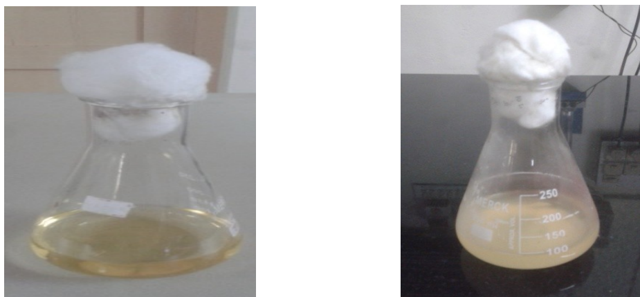
Figure 4.91 (a) Representative photograph of the 24h grown cell free supernatant of strain 8S1 (b) photograph of \text{TiO}_2 -NPs synthesized using 24h cell free supernatant of strain 8S1
