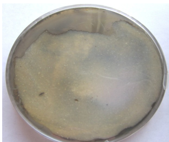
Figure 4.40 (a): Formation of clear zone indicating the reduction of \text{AgNO}_3 in the medium (b) Silver coating on the agar plate indicating formation of AgNPs
