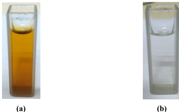
Figure 4.81 Representative photograph showing the change in colour of the AgNPs colloidal solution (a) Before the addition of \text{HgCl}_2 solution (b) After addition of \text{HgCl}_2 solution
