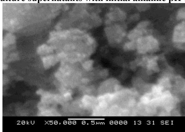
Figure 4.100 SEM image of TiO 2 -NPs synthesized using 6S1 bacterial cell free culture supernatants with initial alkaline pH 11
