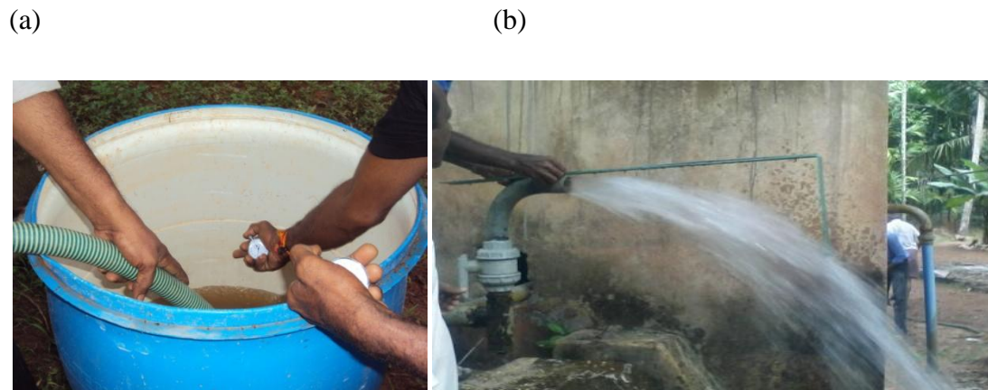
Fig. 3.9 Discharge measurement in the field using (a) collecting tank (b) trajectory methods
