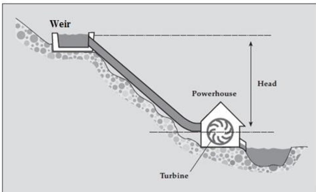
Figure 6.8: Measurement of head in a hydropower station(Sale Michael et al. 2006)
