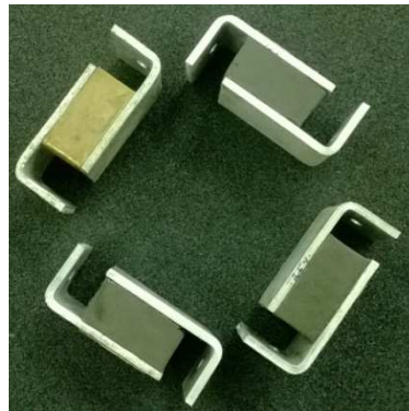
Figure 3.6 Test samples for forced-vibration transmissibility tests
