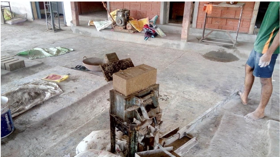
Fig. 7.6 Ejecting the soil block after compression process
