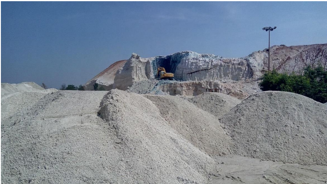
Fig. 1.2 Profile of granulated blast furnace slag at Kirloskar Ferrous Industries Limited, Koppal, Karnataka, India
