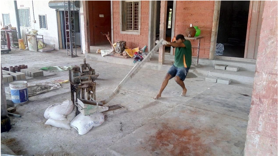
Fig. 7.5 Compressing the block by pulling down the lever arm
