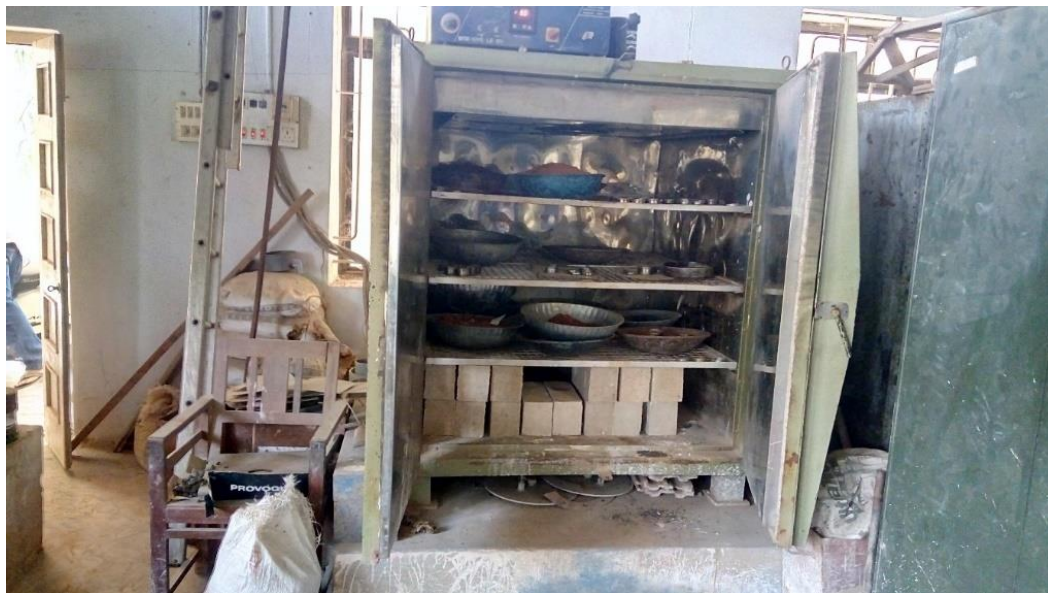
Fig. 7.9 Placement of soil blocks in hot air oven for water absorption test.
