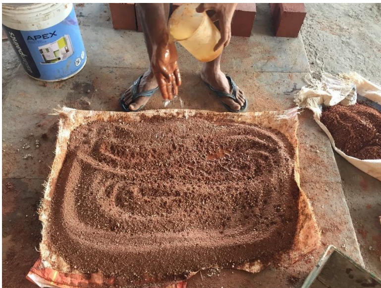
Fig. 7.4 Addition of water to the dry mix
