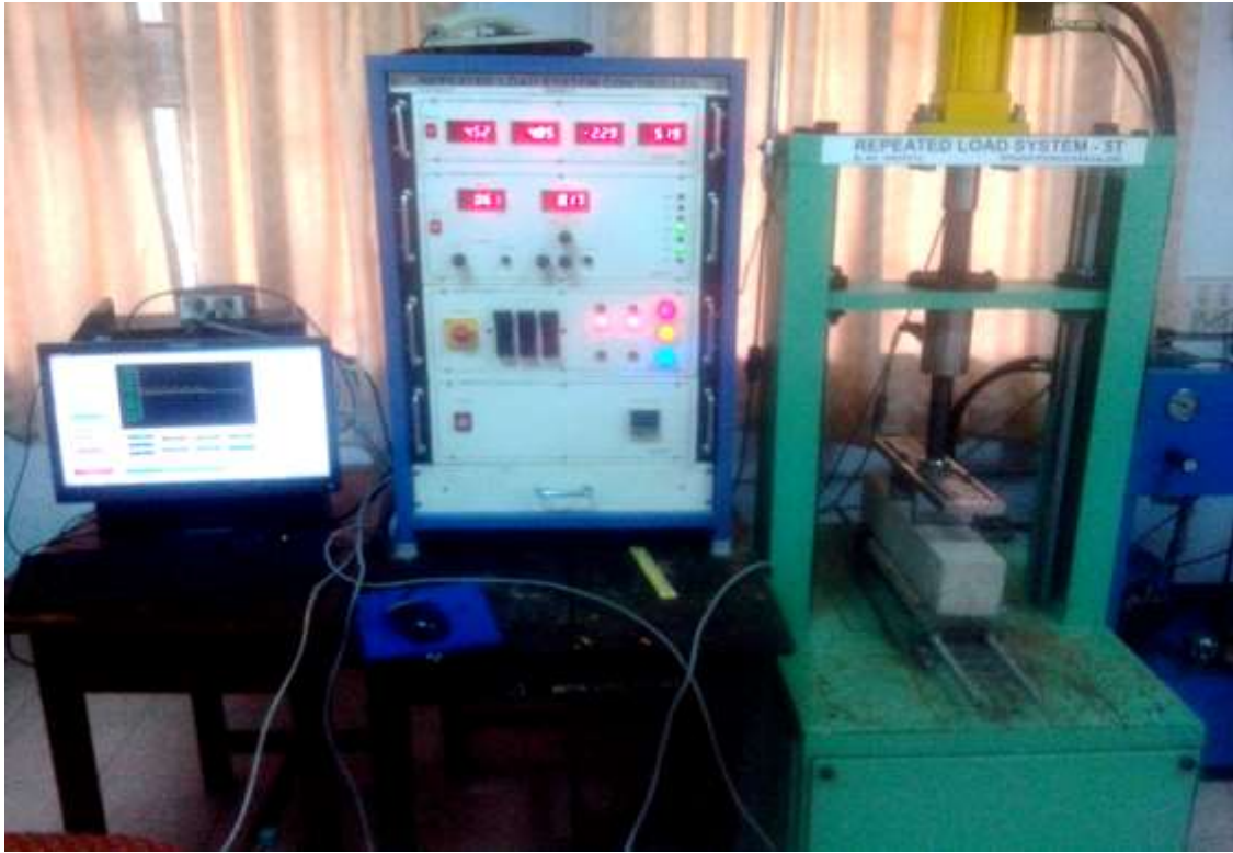
Fig 3.2 Flexural fatigue testing setup
