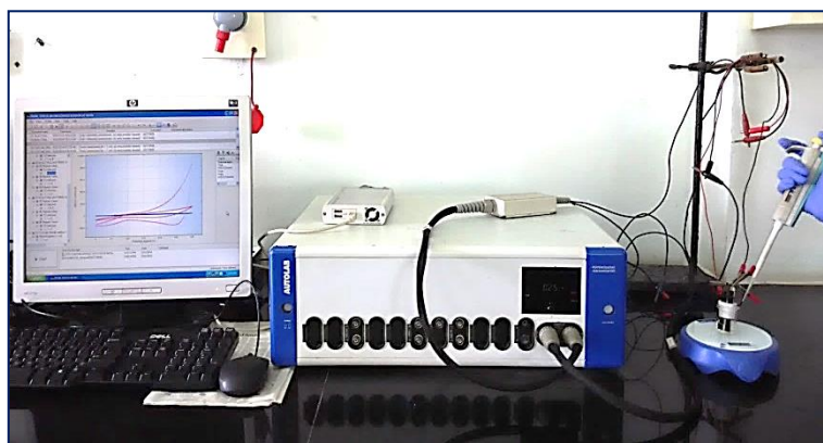
Figure 3.3 Electrochemical workstation (AUTOLAB)
