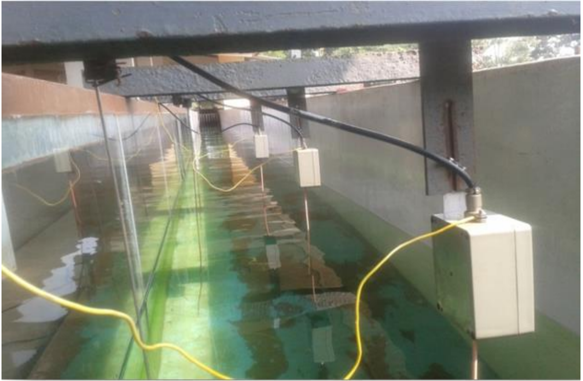
Plate 3.2 Arrangement of wave probes
