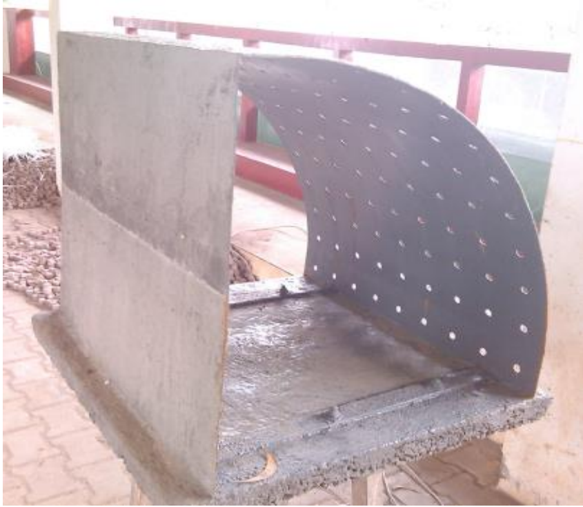
Plate 3.4 QBW model after casting and fixing
