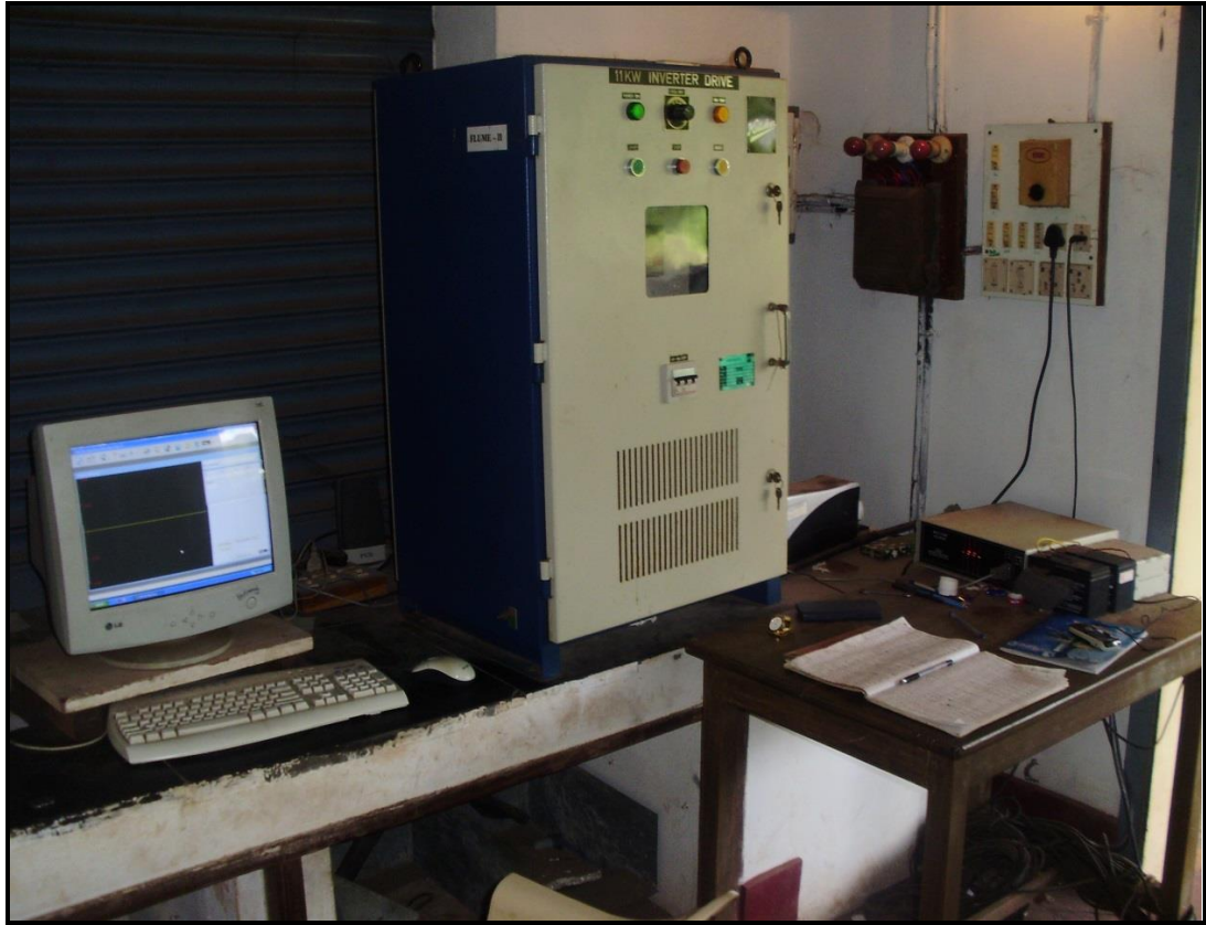
Plate 3.6 Data acquisition system
