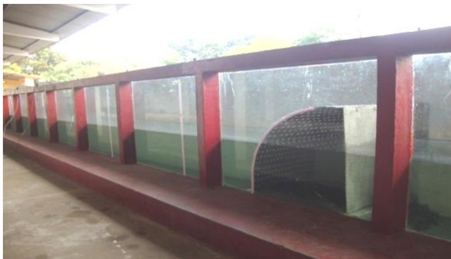
Plate 3.1 A view of wave flume with QBW model
