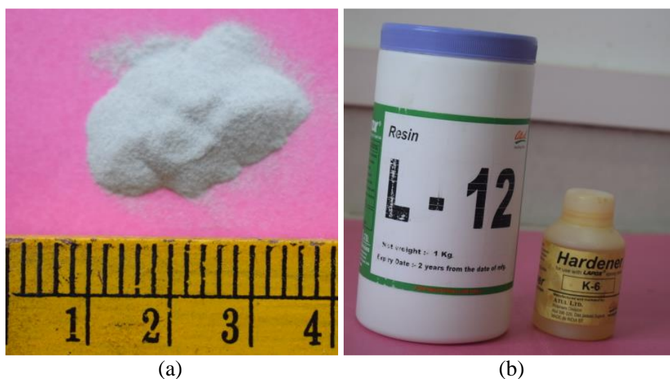
Figure 2.1 (a) Cenospheres and (b) Epoxy resin and hardener used for SF preparation.
