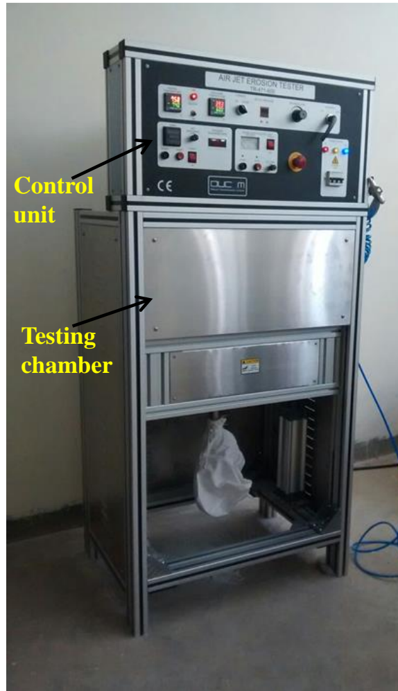
Figure 2.8 Erosion test setup.
