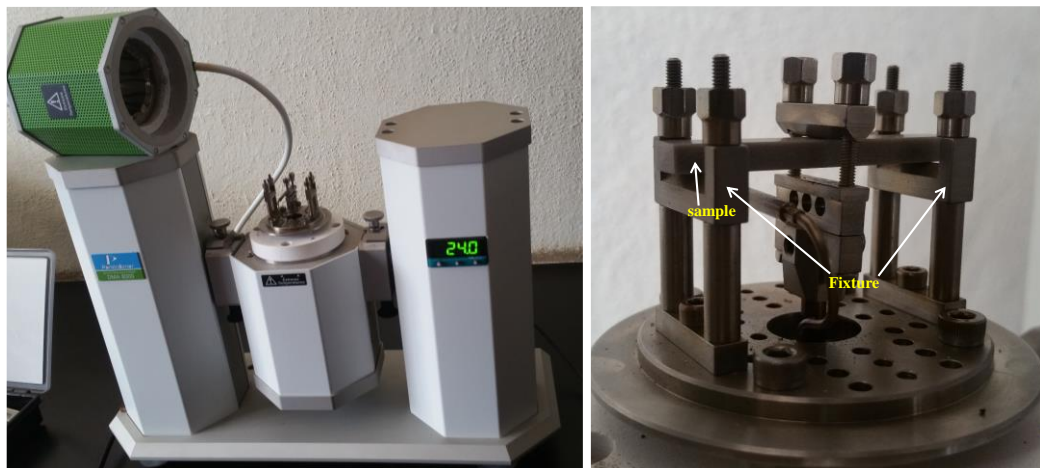
(a) (b) Figure 2.6 (a) DMA setup and (b) Test configuration.
