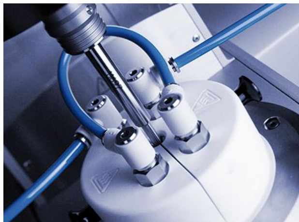
Figure 3.4 Magnetorheological device cell
