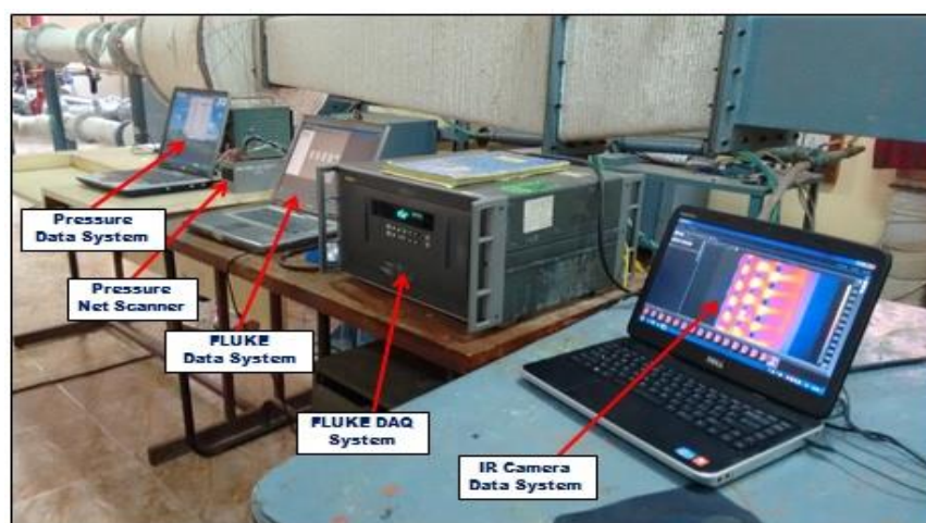
Fig. 3.23 Temperature DAQ system, pressure net scanner and IR instruments
