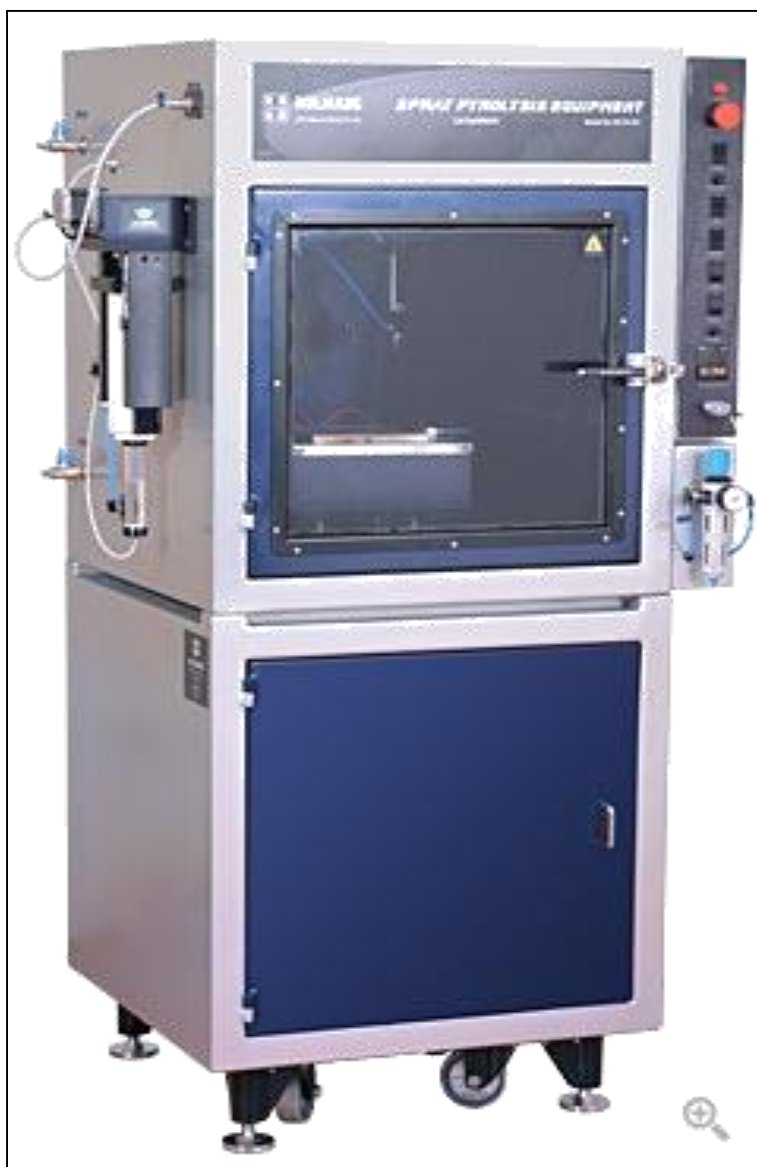
Fig. 2.1 Schematic representation of spray pyrolysis unit.
