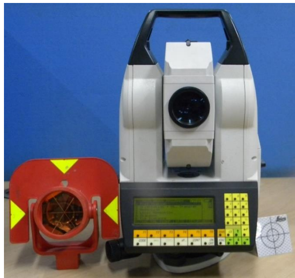
Fig. 3.22 Total station TDA 5005 with reflective targets
