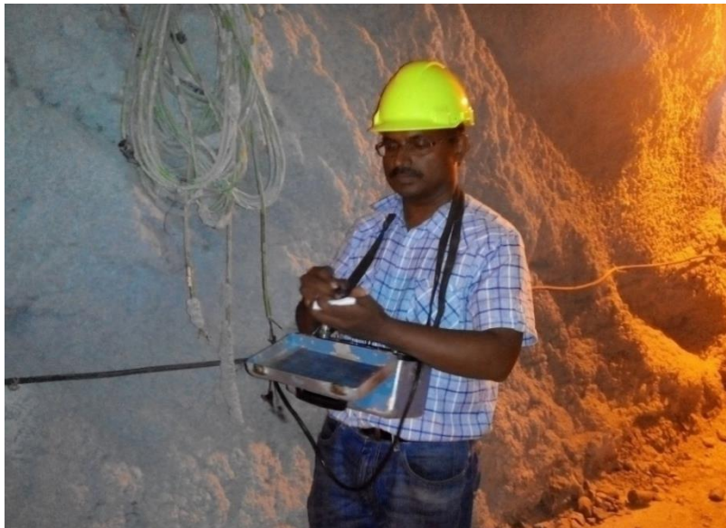
Fig. 3.21 Monitoring of load cells at walls of the cavern
