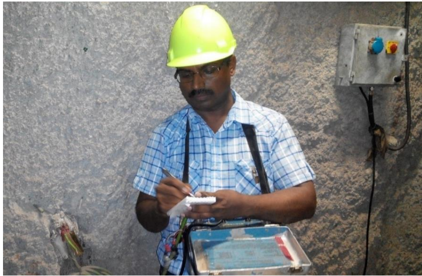
Fig. 3.25 Monitoring of piezometers at walls of the cavern
