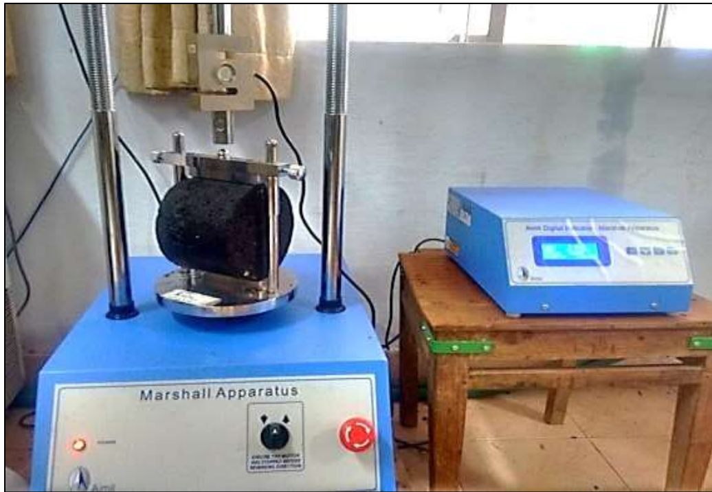
Fig. 3.5. Indirect tensile strength test setup
