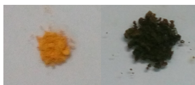
Fig. 4.53 Color change of receptor S2R4 upon dry grinding of receptor S2R4 with 1 equiv. of TBAAcO; S2R4 alone (left), S2R4 + TBAAcO (right)
