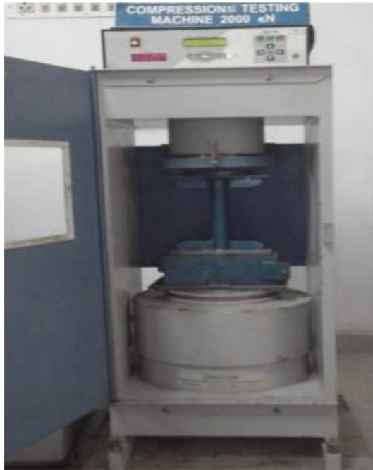
Fig. 2 Application of load for brick compaction
