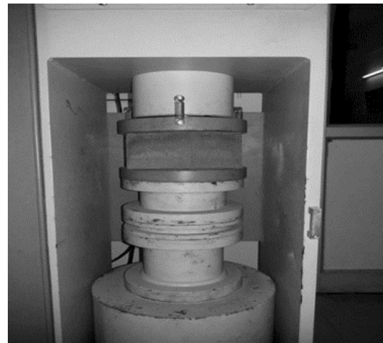
Fig. 5 Testing of bricks for its compressive strength
