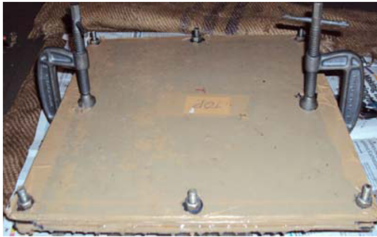
Figure 1 Mould used for casting sandwich samples (see online version for colours)
