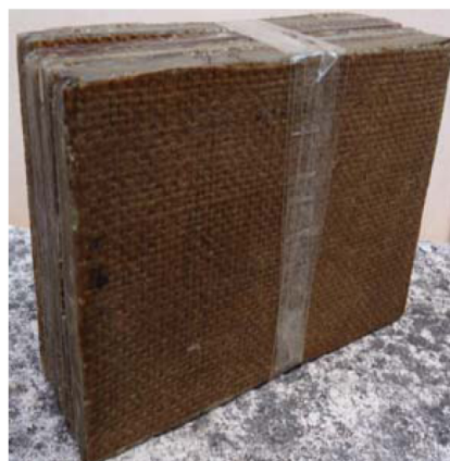
Figure 12 Typical stack of sandwich used for thickness optimisation (see online version for colours)
