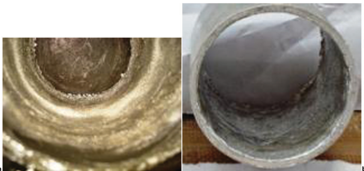
2 Casting of tin of 4 mm thick (teeming temperature: 350°C) at a 600 and b 800 rev min -1
