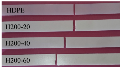
Fig. 10. Representative specimens of neat HDPE and syntactic foams after tensile test at 1.6 \times 10^{-3} \text{ s}^{-1} strain rate.
