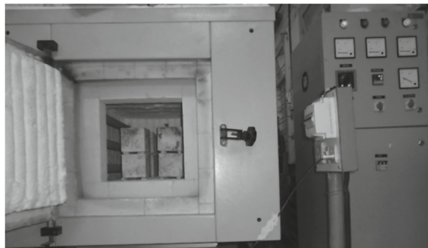
Fig. 1. Muffle furnace and arrangement of specimen for exposure.
