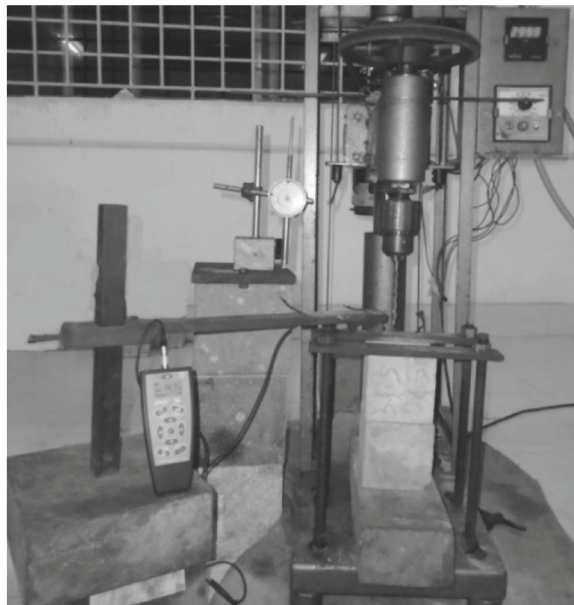
Fig. 5. Test setup for determination of drilling time.
